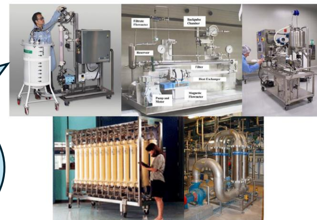
Figure 4.C. Complete cross-flow filtration systems at different process scales. Top row: laboratory/pilot scale. Bottom row: industrial scale.
